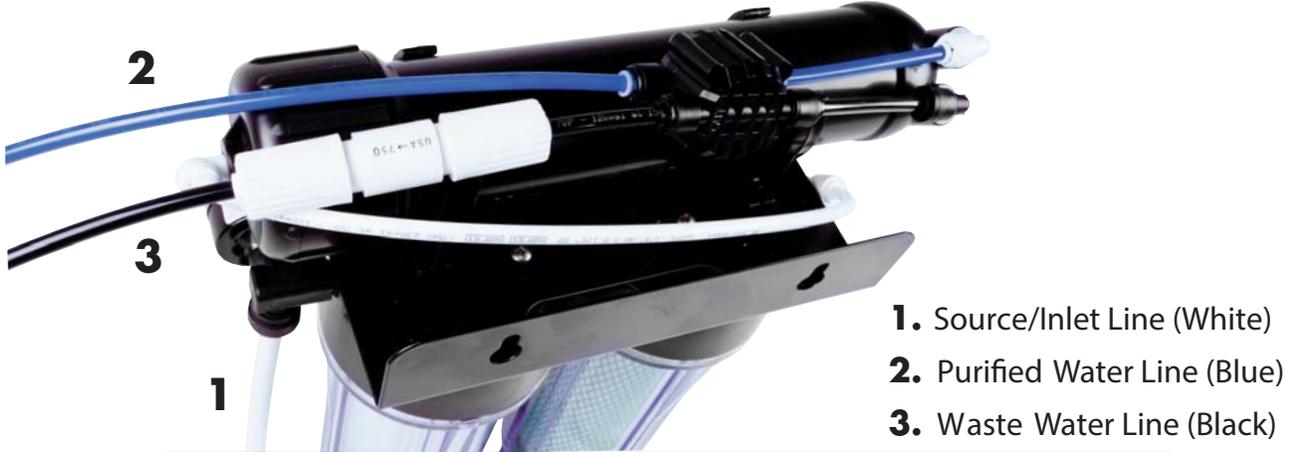
Upon initial start up of system, slowly turn the source water on until both the carbon and sediment filters have water in the housings. Next, open source water up all the way (do not exceed 80 psi). Flush the system for 30-45 minutes when the system is new and/or when you replace your membrane. This will flush out the food grade preservative in the membrane .
